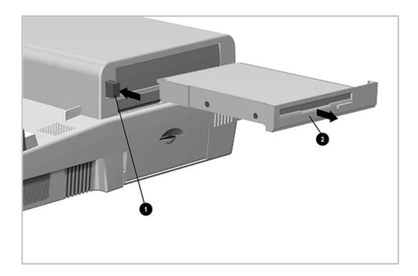
Figure 7-5. Removing a Mass Storage Device
